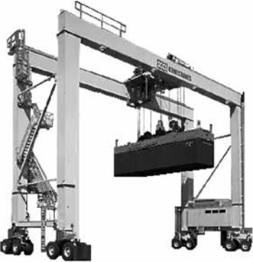
CODE C55 Rubber Tyred Gantry Crane
