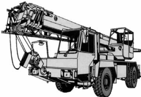
CODE C33 Hydraulic Mobile Crane Up to 50 000 kg capacity
