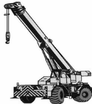
CODE C34 Hydraulic Crane Pickup and Carry up to 50 000 kg capacity
