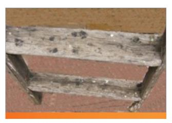
This is what a ladder should not look like. The timber of the rungs is badly worn and obviously unsafe. Remember that the rungs of a ladders should be able to safely support the weight of even a heavy worker.
