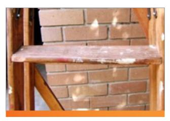
This is what a safe rung looks like. The timber is in good condition and firmly fixed to the frame.
